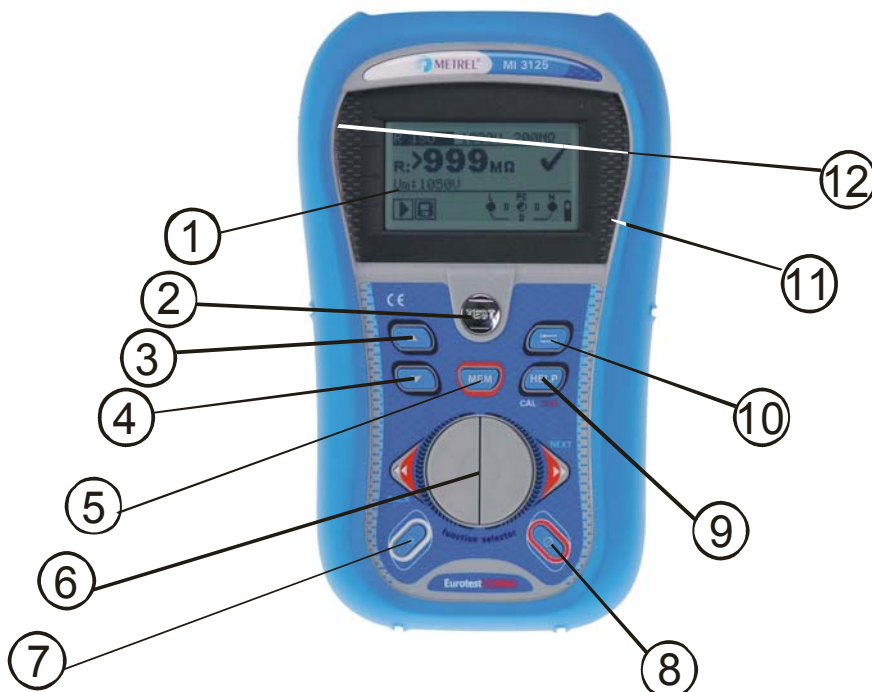
Figure 3.1: Front panel (picture of MI 3125B)
