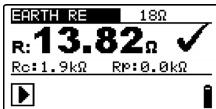
Figure 5.35: Example of earth resistance measurement result
